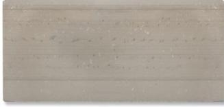
White carbon steel material, CX, with a precision low-friction metallic coating for difficult Flexo and Gravure doctoring applications. This material is not recommended to be used in Flexo containment applications. CXP4 is beneficial when running chrome gravure cylinders with minimal engraving since the coating helps to provide lubrication between the blade and cylinder and reduce haze and streaking issues. The coating will also provide corrosion resistance when used with water based inks
