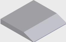
A beveled edge shape with a nominal 4.5° bevel angle. The long bevel provides effective tip deflection and contact angle control under applied blade loading forces with minimal tip growth as the blade wears
